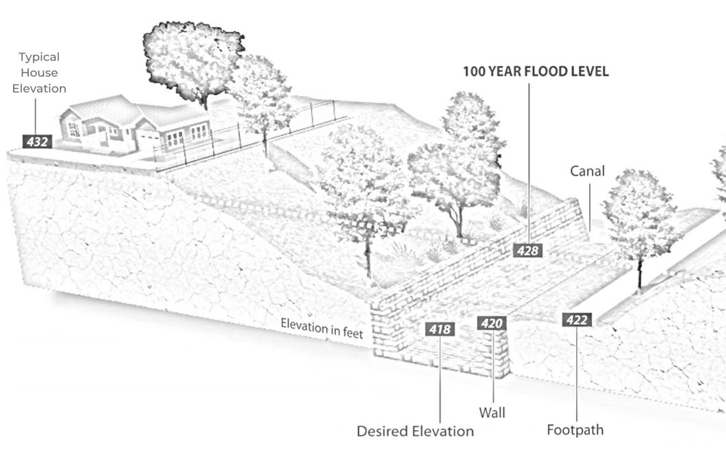
The houses in Valley Ranch are built at a higher elevation so that when it rains, water stays close to canals and away from homes.
